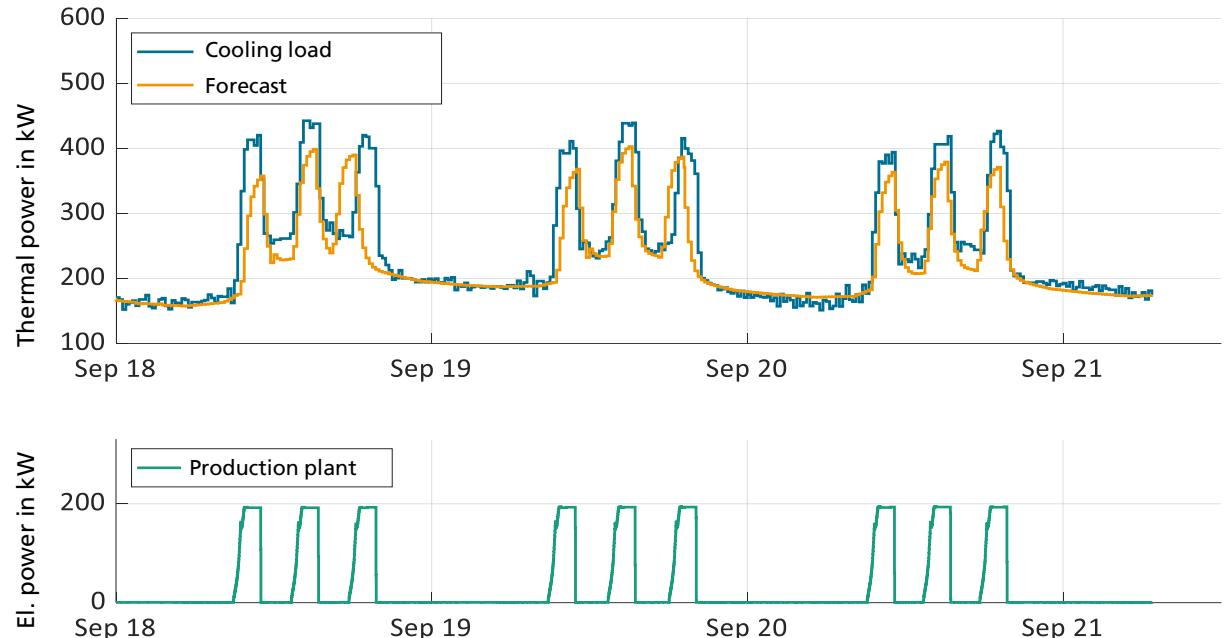
Forecast of cooling load (top), which is strongly shaped by the operation of a production plant (bottom)
