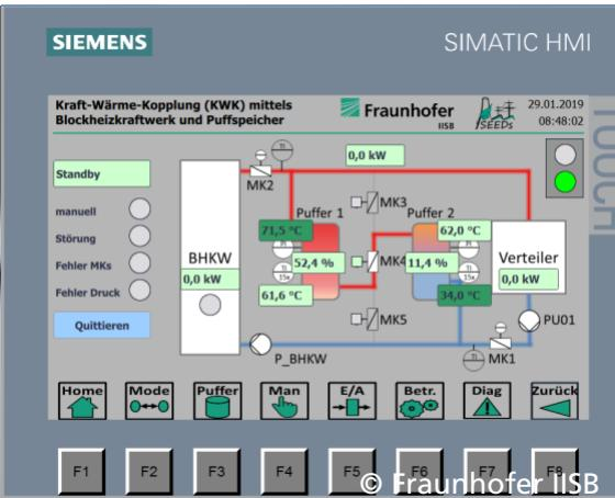
Overview screen for visualization of a CHP plant (HMI)
