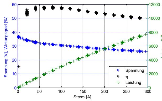
Measurement data of a fuel cell experiment
